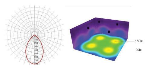
Aquaray 5 shown in a typical room (5x5m) wit h a ceiling height of 2.4m
